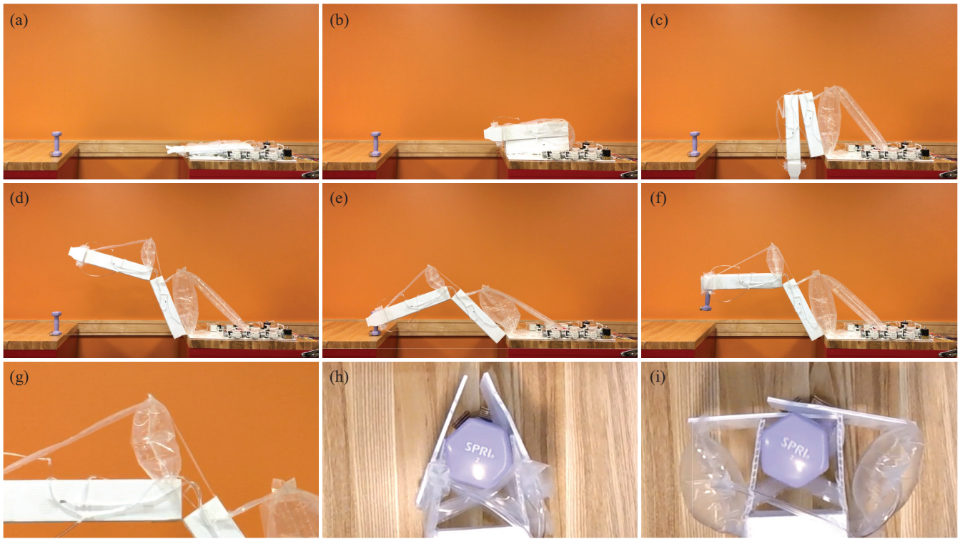
Fig. 10: The arm (a) in its flat configuration, (b) self-folding, (c) upright, (d) reaching out, (e) grasping, (f) lifting. (g) The elbow pouch. The gripper (h) in position and (i) grabbing a dumbbell.
