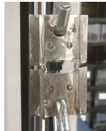
FIGURE 4: TENSILE TEST FOR MEASURING YOUNG'S MODULUS OF THE HYDROGEL.
