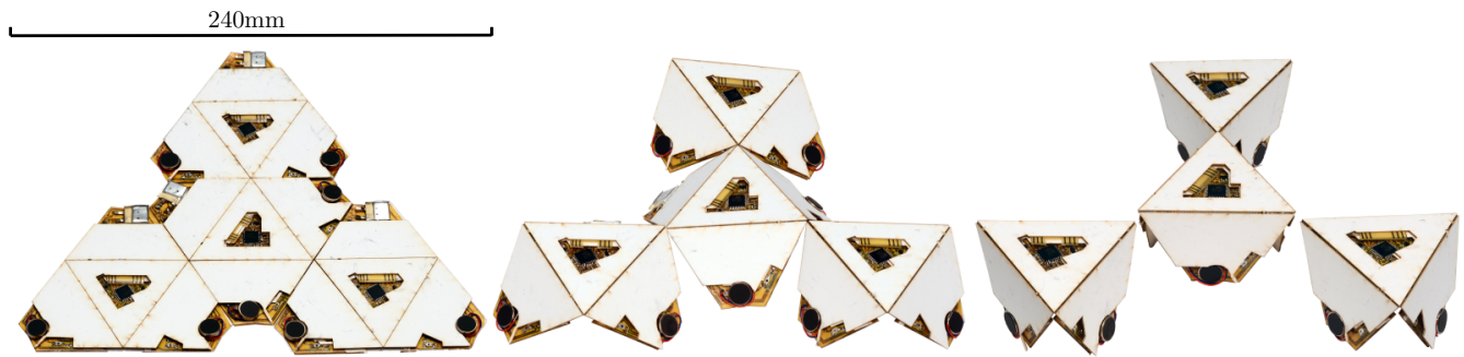
Fig. 12: (Left) A collective of four robots is fabricated as a single composite held together by one monolithic sheet of SMP. (Middle) Individual robots autonomously detach from one other by joule-heating the SMP connecting them, then self-fold their legs, standing up in the process. (Right) Self-folded robots use vibration motors and embedded phototransistors to navigate by phototaxis.
