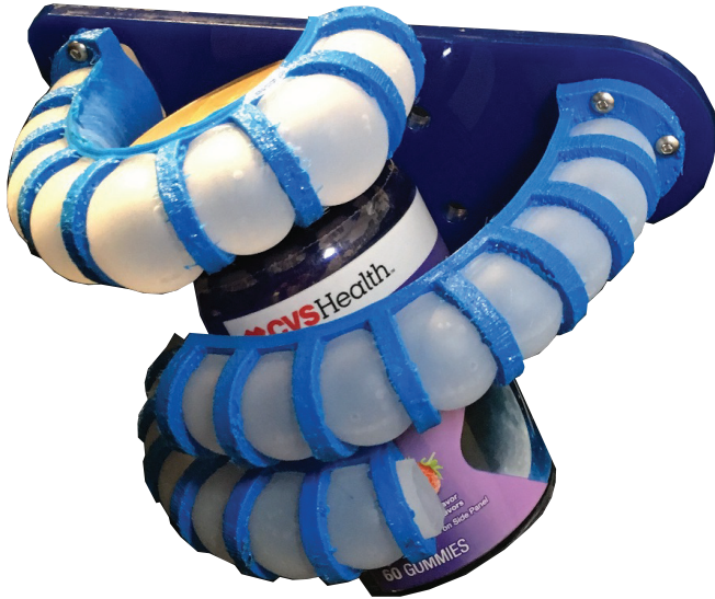
FIGURE 1: A gripper composed of soft bending actuators using a hybrid fabrication method with casting and additive manufacturing
