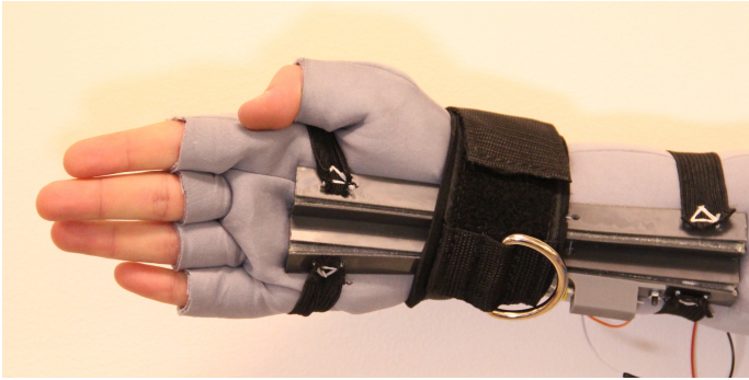
FIGURE 1: Wrist brace design based on a self-folding hinged structure.
