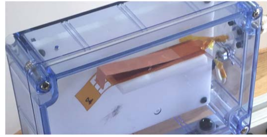
Figure 4. Experimental setup for measuring angular displacement.
