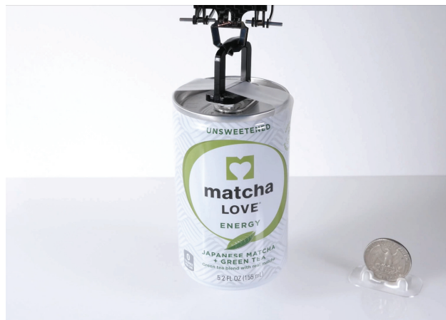
Fig. 12. The wrap gripper lifted a 184 g tea can, the maximum payload demonstrated by these prototypes.
