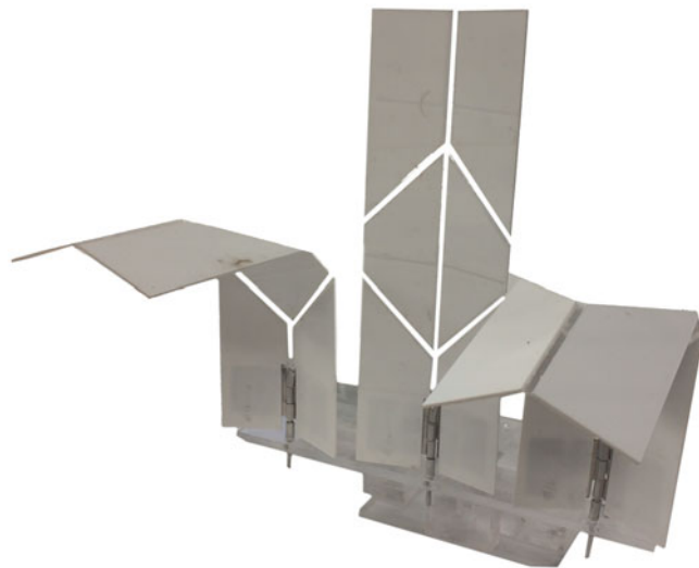
Fig. 1. An origami gripping system with three fingers in different configurations.
